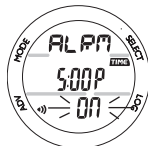
Fig. 21 - DAILY ALARM STATUS
