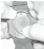
Fig. 120 - BATTERY COVER REMOVAL (without tool)
