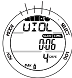
Fig. 89 - VIOLATION GAUGE SURFACE
