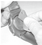
Fig. 119 - BATTERY COVER REMOVAL (using tool)
