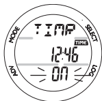
Fig. 101 - CDT ON/ RUNNING
