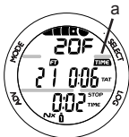
Fig. 82 - DECO STOP MAIN
