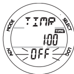
Fig. 110 - FREE CDT STATUS (OFF/READY)
