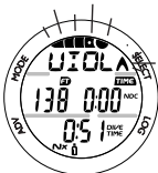
Fig. 88 - VIOLATION GAUGE MAIN
