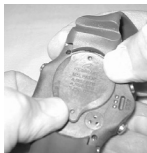
Fig. 124 - BATTERY COVER O-RING (without tool)
