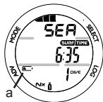
Fig. 3 - LOW BATTERY WARNING
