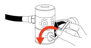
Please screw in the coupling of a high pressure hose to H.P. port and turn it clockwise with a spanner to tighten it. Tightening torque is 9.8 N·m (100kgf·cm).
