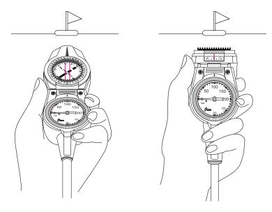
Check the angle of a direction of target with an angle index or the side window, and memorize it. Also, match an index mark with the head of magnetic needle on a compass disc.
