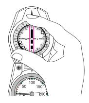
After an entry, hold the compass correctly, and turn your body to adjust direction so that the lubber's line may be maintained at the angle which is checked and memorized.
