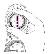
After an entry, hold the compass correctly, and turn your body to adjust direction so that the head of magnetic needle may be maintained at the position of the index mark or the index of the side window matches the angle decided.
