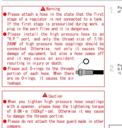
Please remove the plug from the H.P. (high pressure) port of the first stage of a regulator.
