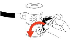
Please screw in the coupling of a high pressure hose to H.P. port and turn it clockwise with a spanner to tighten it. Tightening torque is 9.8 N • m (100kgf • cm).
