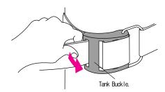
Draw a belt through the slot of the tank buckle.
