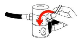
Please screw in the coupling of a B. C. hose to L. P. port and turn it clockwise with a spanner to tighten it. Tightening torque is 9.8 N·m (100 kgf·
