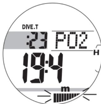
1. Oxygen accumulation (O<sub>2</sub>) and partial pressure of oxygen (PO<sub>2</sub>) bar graph flash, and at the same time, the dot display shows the letter of "PO<sub>2</sub>".
